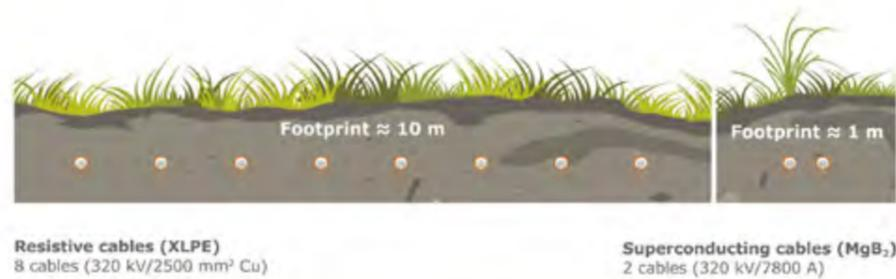
Fig. 8. Comparison of the environmental footprint of resistive XLPE cables and MgB<sub>2</sub> superconducting cables for a 6.4 GW DC power link.
