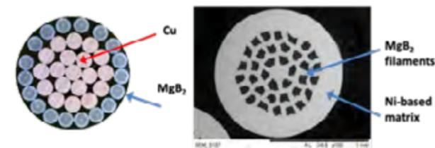
Figure 2. Picture of the 10 kA cable conductor consisting of 18 MgB<sub>2</sub> wires wound around a copper core (left) and one MgB<sub>2</sub> wire composed of 36 superconducting filaments embedded in a matrix of nickel and monel (right).
