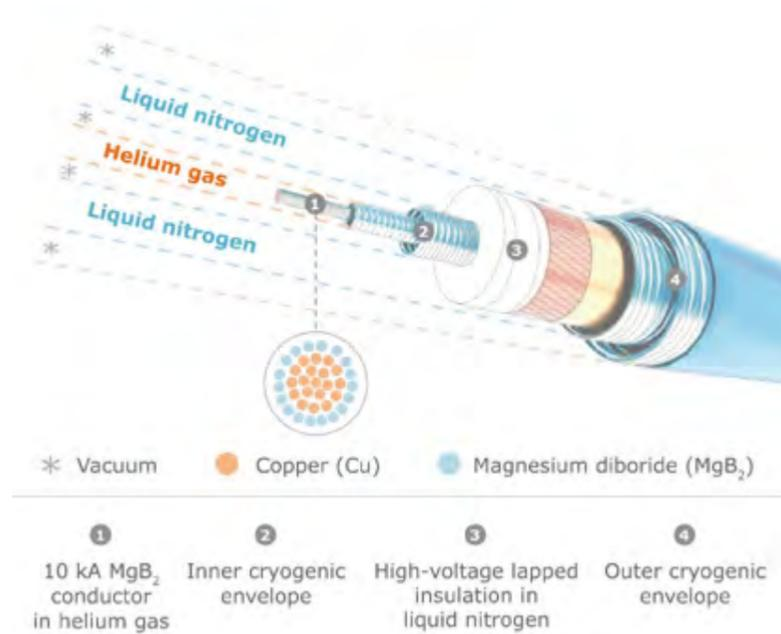
Figure 1. Sketch of the 3.2 GW MgB<sub>2</sub> cable system showing the key components. The electrical terminations are not represented here.
