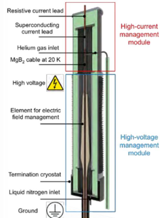
Fig. 5. Sketch of the HVDC termination developed for Best Paths, highlighting its modular design.
